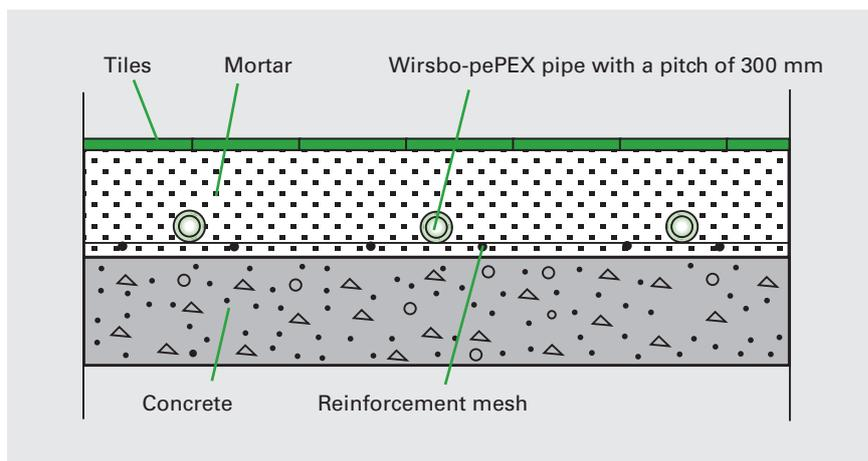
Here the pipe loops are set in mortar screed above concrete.
