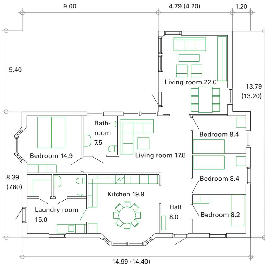
Figure 24 House: architect's drawing
