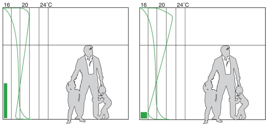
Figure 4 Radiator heating temperature curve (left) and figure 5 Convector heating temperature curve (right)
