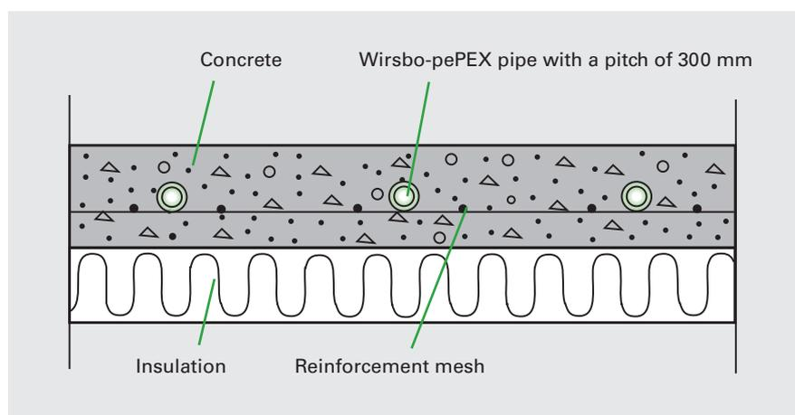
Figure 9 Concrete floor with insulation underneath. The pipe loops are laid on a mesh and fixed with tying wires before concreting.
