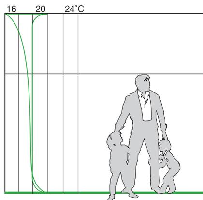
Figure 3 Underfloor heating temperature curve
