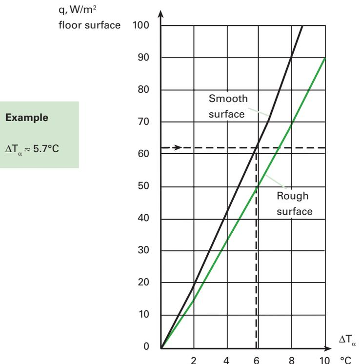
Diagram 5 Heat exchange, floor surface
