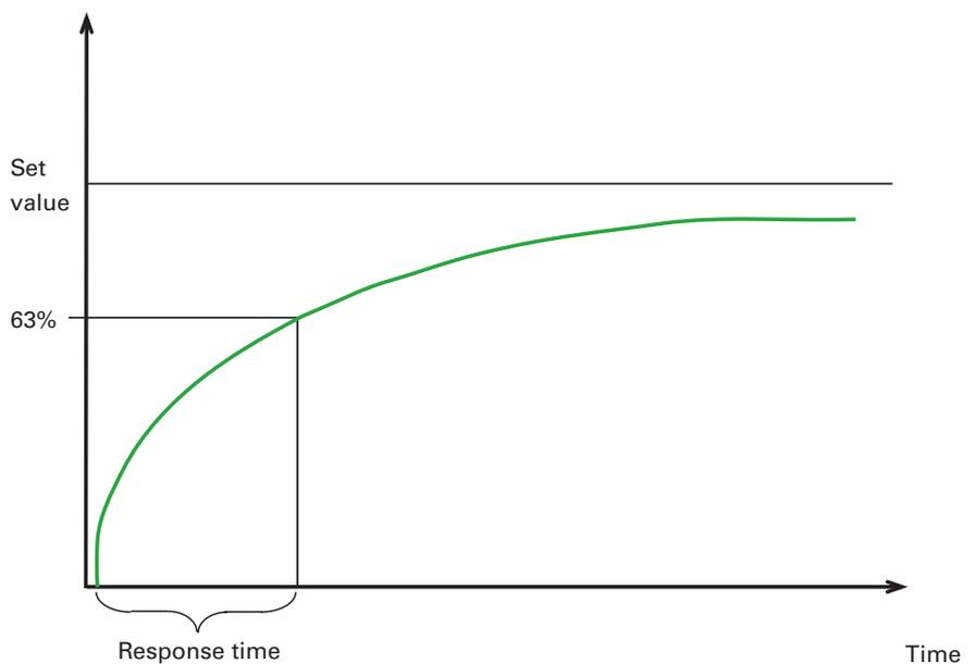
Figure 19 Typical response time diagram.
