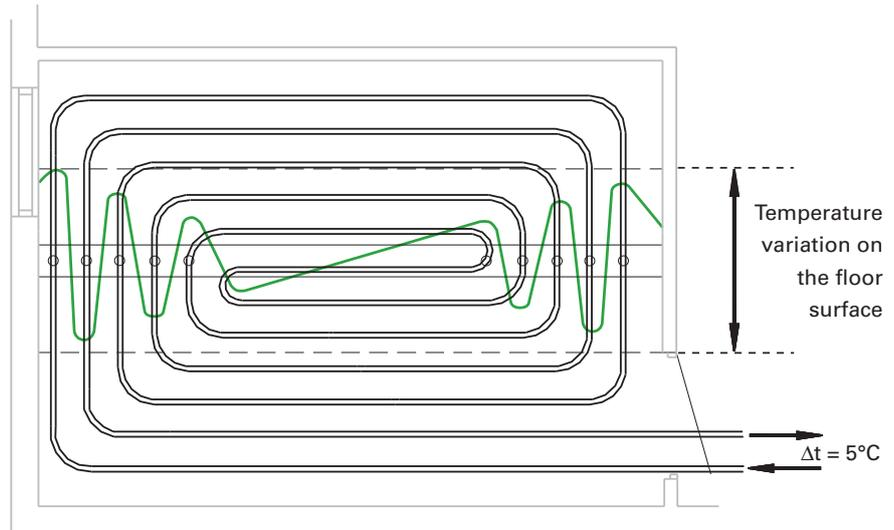
Figure 22 Configuration C, supply and return pipes in a parallel run: helical arrangement
