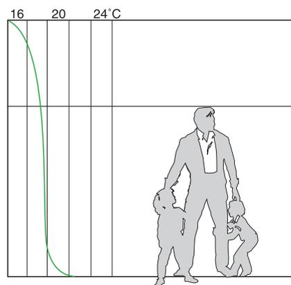
Figure 2 Ideal heating temperature curve
