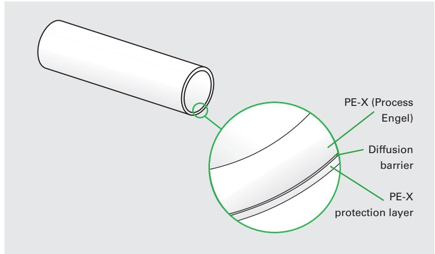
Figure 8 Oxygen barrier on a Wirsbo-pePEX pipe
