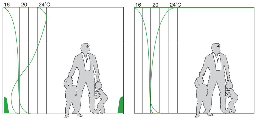
Figure 6 Forced air temperature curve (left) and figure 7 Ceiling heating temperature curve (right)
