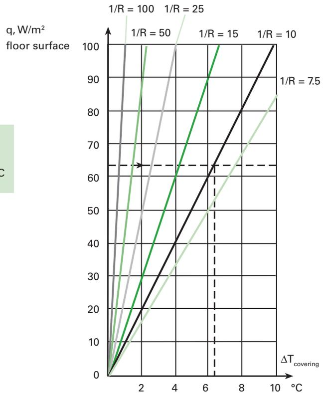
Diagram 6 Temperature drop through floor covering material
