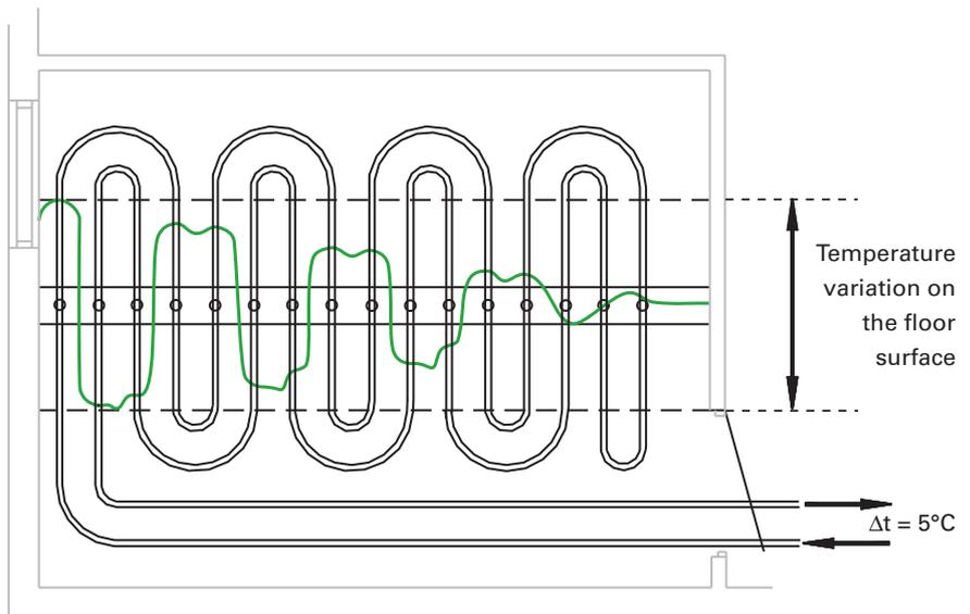
Figure 21 Configuration B, supply and return pipes in a parallel run
