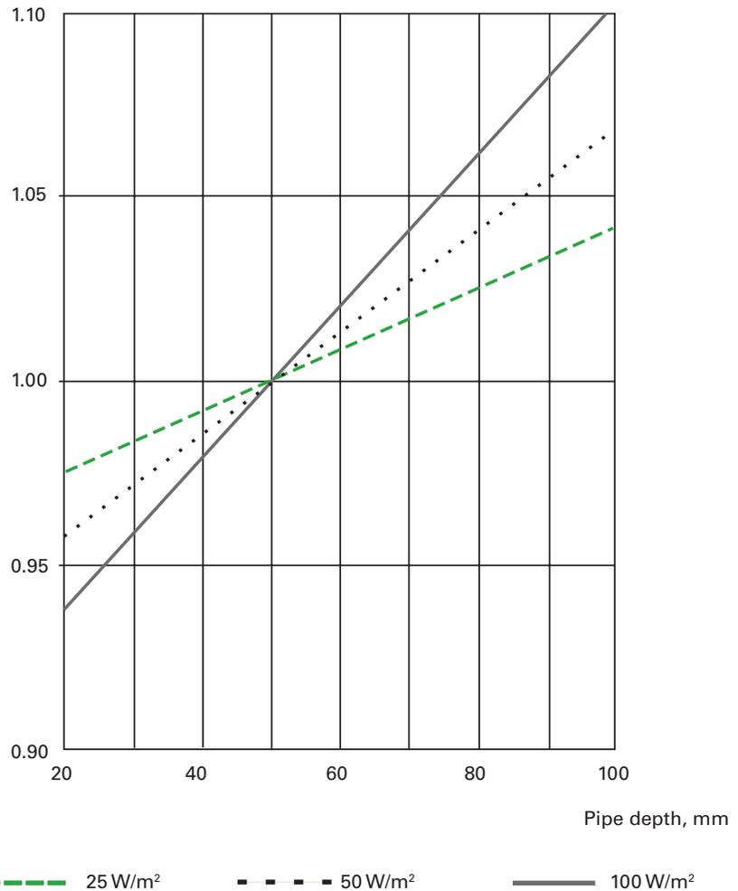
Diagram 2 Water temperature as a function of pipe depth
