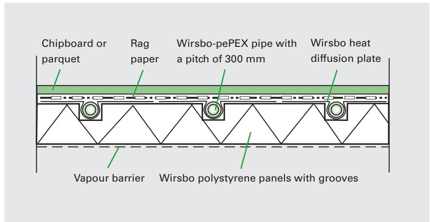
Figure 14 Cross section of a floating floor
