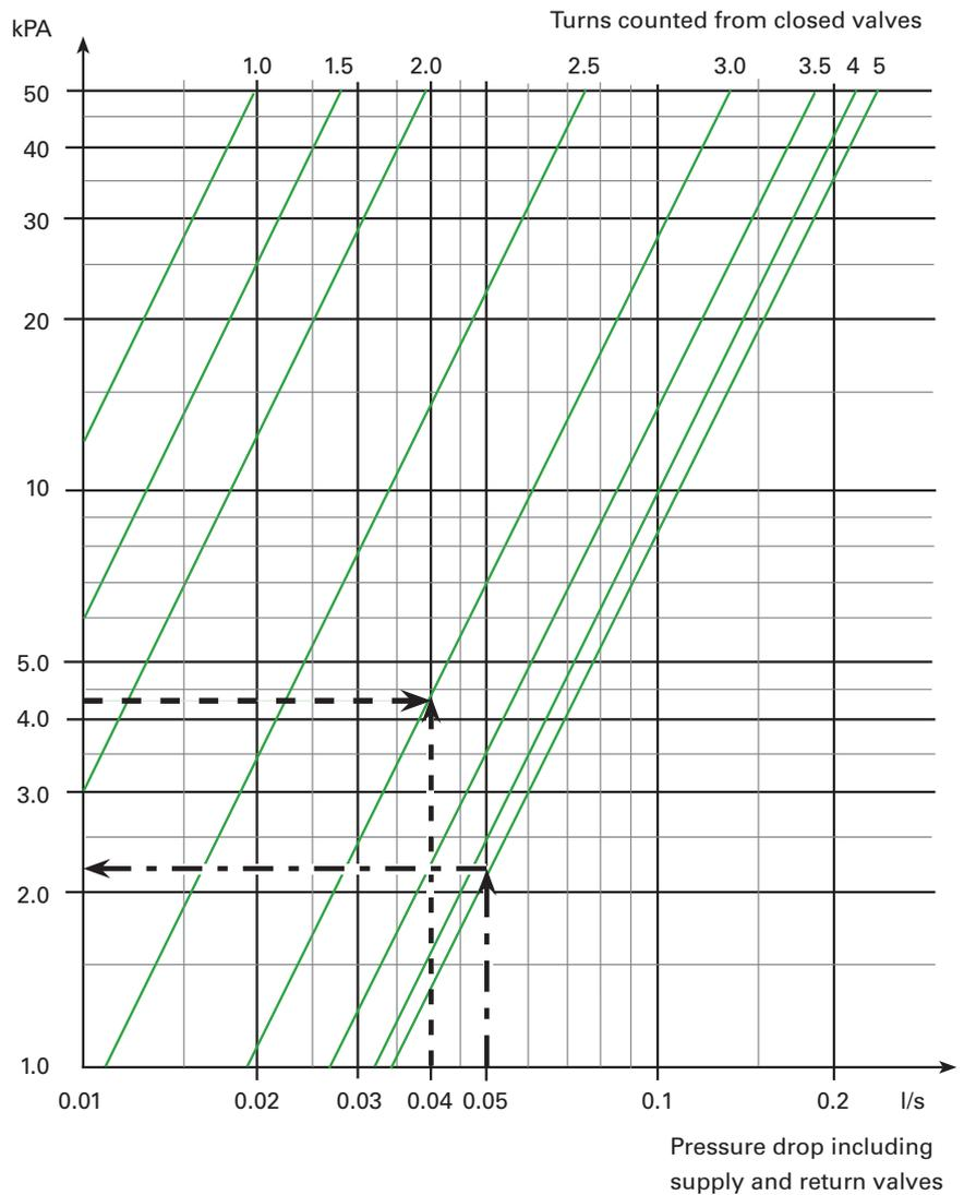
Diagram 8 Manifold valve chart
