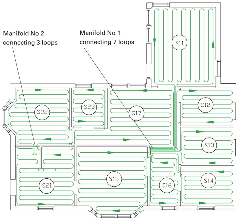
Figure 26 House drawing with pipe loops and manifolds
