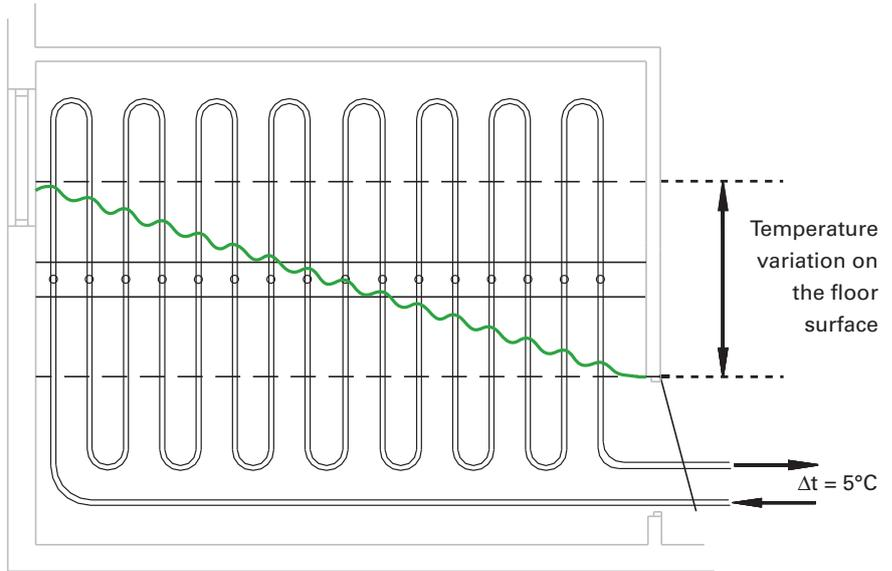
Figure 20 Configuration A, single serpentine run
