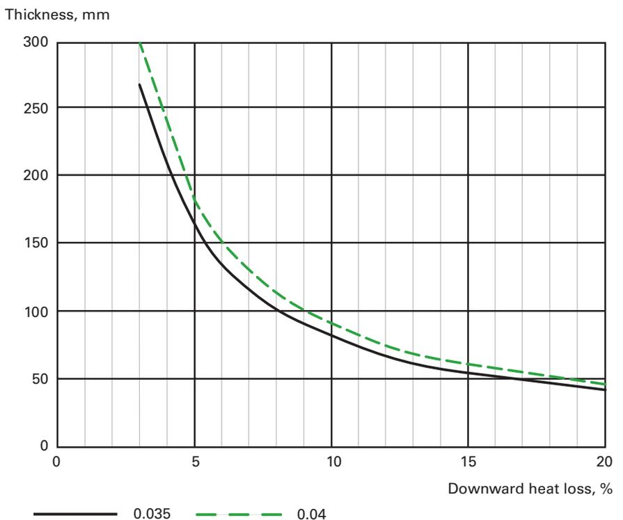
Diagram 10 Insulation thickness
