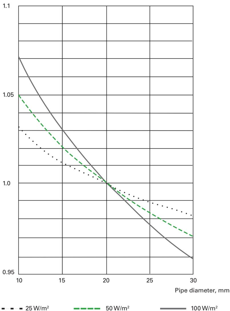
Diagram 1 Water temperature as a function of pipe diameter
