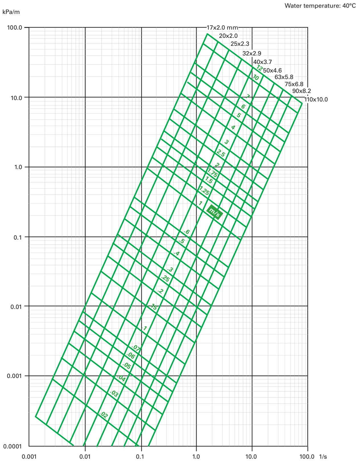
Diagram 9 Pressure drop nomogram Wirsbo-pePEX and Wirsbo-evalPEX
