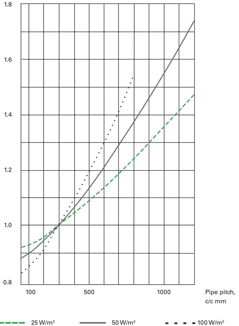
Diagram 3 Water temperature as a function of pipe pitch
