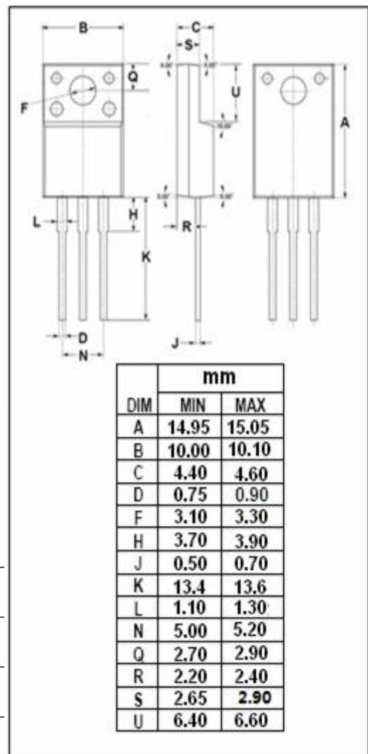
**Isc N-Channel MOSFET Transistor**
